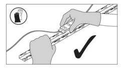
boxLED mounting profile insert module
