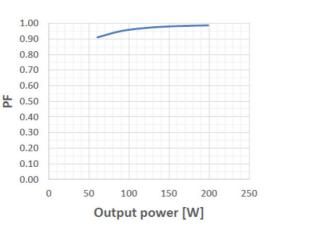
OT 200 2DIM NFC IP67 Typical Power Factor vs. Load
