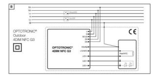
OT 4DIM NFC G3 Wiring Diagram I
